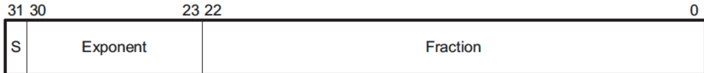
Figure 2-1 Single-precision data format
